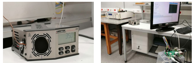
Figure 5. Black body calibration setup
